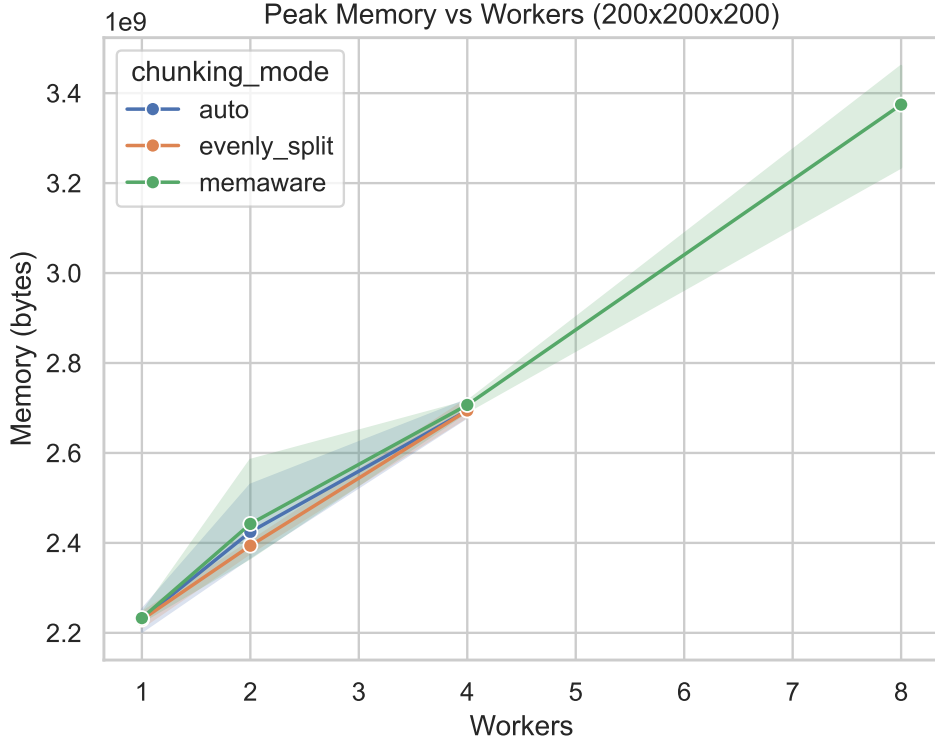
Figure 3. Peak memory usage comparison for a 200 \times 200 \times 200 volume. Memory-aware chunking maintains consistent memory usage below the safety threshold across all worker counts, while auto and evenly-split approaches show increasing memory consumption that leads to OOM failures beyond 4 workers.
