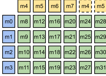
Figure 2. Representation of register utilization by 4x6 kernel.
